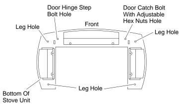
Figure 9 - Locating Threaded Holes for Legs and Door Attachment
